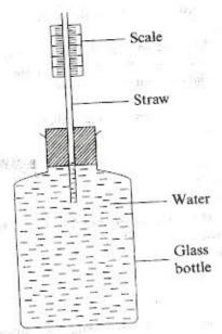
Which one of the following improvements would make the instrument measure smaller changes in temperature?
